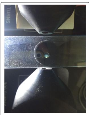
**Fig. 5** Shows polarization of the magnetic nanoparticles under the influence of 0.7 T electromagnetic field.
