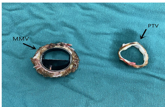
Fig. 1 Physical drawing of a dismantled bileaflet mechanical valve. When the mechanical valve was removed, one lobe of the valve was missing, and the proliferative tissue around the valve had a complete annular structure. MMV: Mechanical mitral valve; PTV: Proliferative tissue of valve
