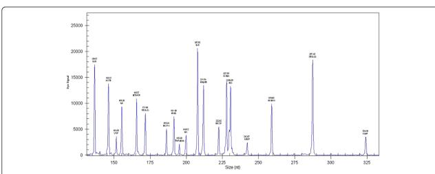
**Figure 2 Multiplex primer RT-PCR capillary gel electrophoresis results before and after optimization.** Multiplex primer RT-PCR capillary gel electrophoresis results after optimization. Multiplex primer RT-PCR capillary gel electrophoresis results before optimization can be found in Additional file 7.
